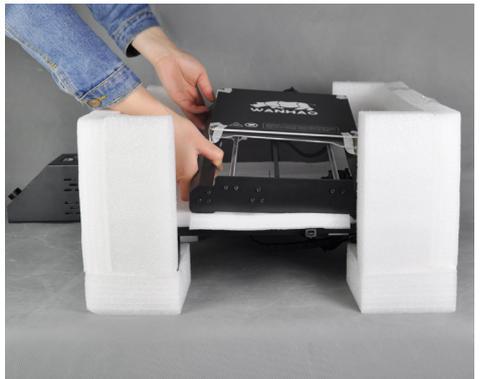
14. Remove the foam on the printer steel frame gently.
