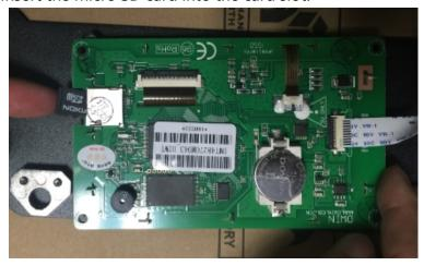
5.9. Turn on the printer. The printer would start flashing automatically. It takes 2.5 minutes to flash the LCD baord. Then the screen would turn black! TURN OFF the printer and UNPLUG the micro SD card.
