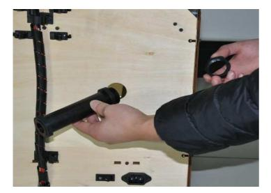
Next, locate your Filament Guide Tube(s). These fit into the tube guide holders at the top of The Duplicator 3's back plate.
