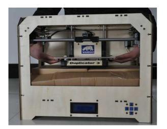
Underneath the build platform you'll see one or two boxes of **Wanhao filament**. Carefully remove these, as well as the remaining packing material. It's easiest if you remove the packing material first.
