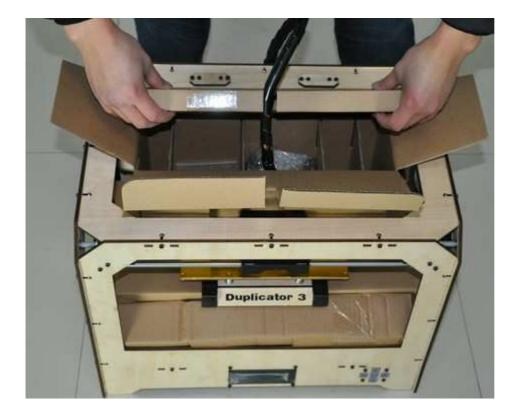
Follow the thick black cable to the Step exstruder MK8. Reach in, grasp the Step exstruder by its sides, and remove it from the
