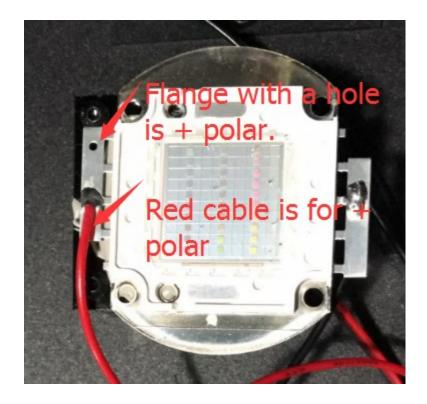
4.3 To use one flat screw driver to bend the + flange up, so the flange and cable would not touch the cooling fin under the light.
