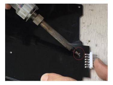
4.3 To solder the new thermistor 2 Pin cable onto the left 2 Pin of connector.
