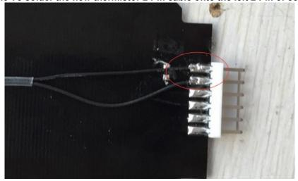
4.4 To stick the thermistor sensor bulb onto the HBP by kapton tape or masking tape. Please handle with care, don't break the bulb.
