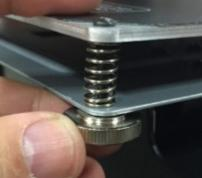
To add the paper card in between the heating bed and spring at 4 corners. You may need to use scissors to trim the card to fit the bed shape.
