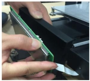
4.4.8. Insert the micro SD card into the card slot.
