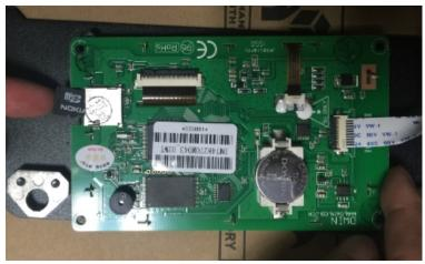
4.4.9. Turn on the printer. The printer would start flashing automatically. It takes 2.5 minutes to flash the LCD baord. Then the screen would turn black! Turn off the printer and unplug the micro SD card.
