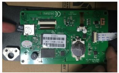
4.4.9. Turn on the printer. The printer would start flashing automatically. It takes 2.5 minutes to flash the LCD baord. Then the screen would turn black! Turn off the printer and unplug the micro SD card.
