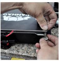
1.3 Repeat 1.1 and 1.2 to replace the rest 3 wing nuts with thumb nuts.
