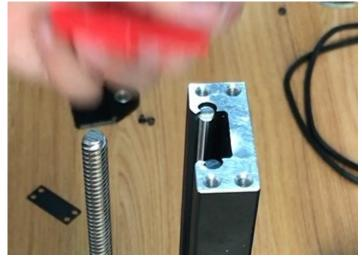
**4.4** Amount the plastic bracket onto the top of track and bolt on M4\*8mm bolt. **Important notice. The stock bolts are M4\*6mm which is not long enough, so please get bolt M4 \*8mm locally or ask WANHAO.**
