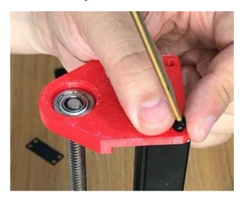
**4.5** The spring couple is not compulsory. If the plastic bracket has already correct the wobble issue. You don't have to install spring couple. In case the lead screw is bending hugely, you can install the spring couple to offset the bending.
