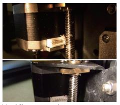
Metal Sheet amount is easy to deformed in shipping.
