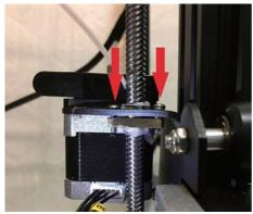
2 bolt bushing could be loose in shipping
