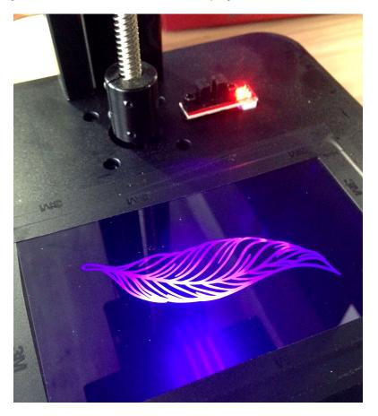
If the image does not appear on screen you should find the root in LCD screen itself or LCD board.
