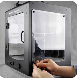
12. Put one of the rop cover on the printer aiming at the hole on the two sides.
