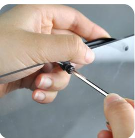
6. Fix the front cover on the printer with the 2.5mm hex wrench and another four M4\*16 screws.
