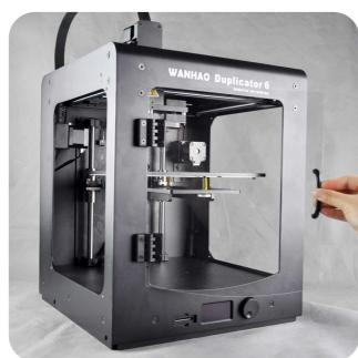
9. Fix the side cover with the 4mm hex wrench and M5\*10 screw. **NOTE:** You should not fix the first three screws too tight at first.
