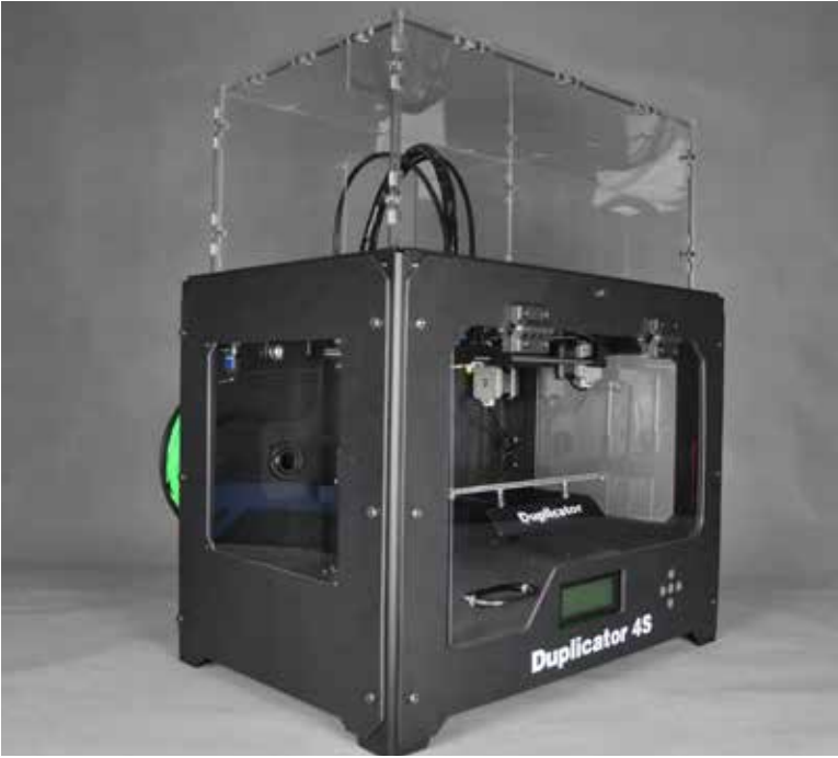
Full covered heating chamber, No curving in ABS printing
