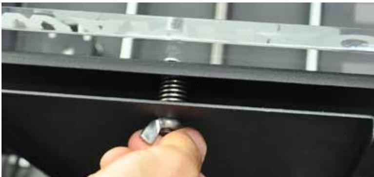
6. Insert one name card between the nozzle and plate(0.1mm thick)
